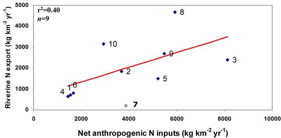
Figure 7. Export of TN at each sampling station versus net anthropogenic inputs in each sub-catchment. Net input is defined as the sum of anthropogenic inputs minus the N exported from the basin as agricultural products. The value from sub-catchment 7, marked with an open diamond (◇), was not included in the regression analysis.
